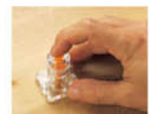
Plunger JUMPS when passed over fasteners.
