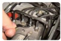
With 6 point, straight slot, reinforced design, offset, for brake line screw fittings
