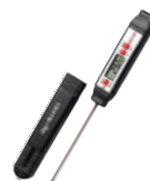
MET450L PEN TYPE DIGITAL MULTI-STEM THERMOMETER TEMPERATURE RANGE : -50°C TO 300°C, -58°F TO 572°F RESOLUTION : 0.1° FOR -19.9° TO 199.9°, OTHERWISE 1°
