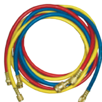
R134a CHARGING HOSE WITH 1/2" ACME x 14mm FITTINGS YELLOW : 1/2" ACME (F) x 1/2" ACME (F) BLUE & RED : 1/2" ACME (F) x 14mm (M)
