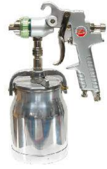
TS-1091 H.V.L.P. Air Spray Gun With 1,000cc Aluminum Cup & 1.7mm Nozzle
