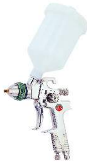
TS-1004 H.V.L.P Air Spray Gun With 600cc Nylon Cup & 1.4mm Nozzle
