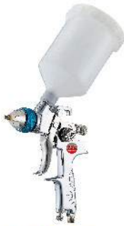
TS-2002G H.V.L.P Air Spray Gun With 600cc Nylon Cup & 1.4mm Nozzle
