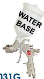
TS-1031G H.V.L.P Air Spray Gun With 600CC Nylon Cup & 1.4mm Nozzle
