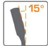
15° offset box end for knuckle clearance.
