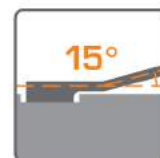
15° offset box end for knuckle clearance.
