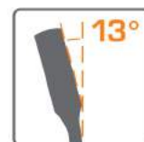
13° offset flare nut drive for knuckle clearance.
