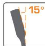
15° offset flare nut drive for knuckle clearance.
