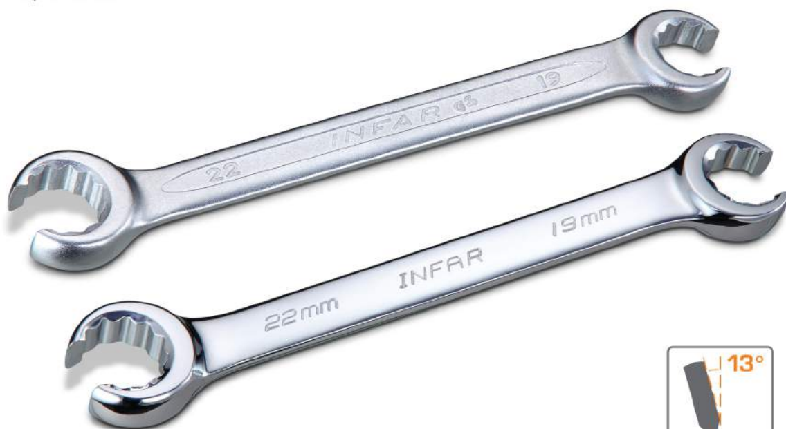
13° offset flare nut drive for knuckle clearance.
