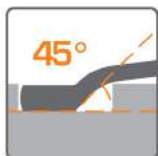
45° offset box end for knuckle clearance.
