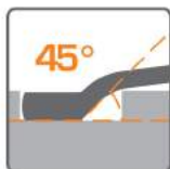
45° offset box end for knuckle clearance.
