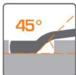
45° offset box end for knuckle clearance.
