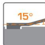
15° offset box end for knuckle clearance.
