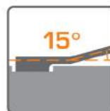
15° offset box end for knuckle clearance.
