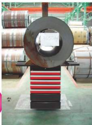
Loading Test 3650KGS(Front)
