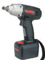
ATI103V 18v 1/2" CORDLESS IMPACT WRENCH VOLTAGE: 18v D.C. SQUARE DRIVER: 1/2" NO-LOAD SPEED: 0 - 2500 RPM MAX. TIGHTENING TORQUE: 2000kg/ cm (144 ft/lb) IMPACTS PER MINUTE: 3300 BPM
