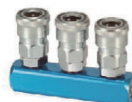
ATH015A MULTIPASS QUICK W/ 3 COUPLER 3 QUICK COUPLE INLET THREAD: 1/4" OUTLET THREAD: 1/4" WORKING PRESSURE RANGE: 0 ~ 150PSI VALVE THREAD: PT (JAPAN STYLE)
