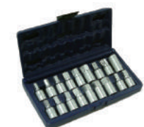
AMR1301I 18PC 3/8" OIL DRAIN PLUG KIT HEX: 8, 9, 10, 12, 14, 17mm; SQ: 7, 8, 10, 11, 12, 13, 14, 5/16", 3/8"; SQ (F) : 10mm; PLUG SOCKET: M16; ∠ : 10mm
