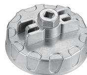
WRF102R OIL FILTER CUP WRENCH (RENAULT) 18 FLUTES x 96mm
