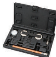
AMT178E PETROL ENGINE SETTING/ LOCKING KIT - VAG 1.2/ 1.4 TFSI & 1.4/ 1.6 FSI - CHAIN DRIVE
