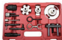
AMR1207E-3 TIMING ENGINE TOOL SET - VAG TDI V6 & V8
