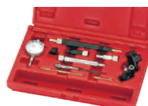
AMM574E-1 8PC TIMING LOCKING TOOL KIT VAUXHALL, OPEL, SAAB, ROVER, XSARA, ISUZU
