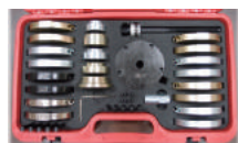
AMR2882E COMPACT WHEEL HUB/ BEARING TOOL SET - VAG CAPACITY: Ø62/ 66/ 72/ 85mm
