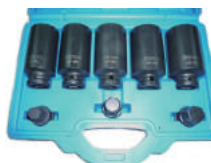
SSR963E-8PC 8PC 1/2"DR. DRIVE SHAFT SOCKET 1/2"DR. HEX: 14/ 17/ 19 x 43mm (L) 1/2"DR. 12PT: 30/ 32/ 34/ 35/ 36 x 85mm (L)
