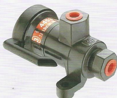
Air Regulator HINO K13C : 44530-1321 ( 7.0~8.5 kg/cm 2 ) 44530-1340 ( 7.5~9.0 kg/cm 2 ) 44530-1360 ( 7.5~8.5 kg/cm 2 )
