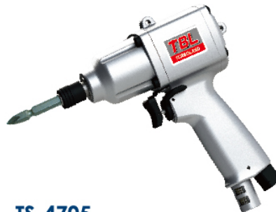
TS-4705 1/4" Heavy Duty Air Impact Screwdriver Max. Torque:44Ft-Lb TS-4705J 1/4" Heavy Duty Single Hammer Mechanism Air Impact Screwdriver TS-4705W/TS-4705JW With 3/8" Square Drive
