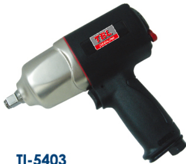
TI-5403 1/2" Composite Industrial Air Impact Wrench(Twin Hammer) Max. Torque:900Ft-Lb
