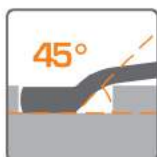
45° offset box end for knuckle clearance.
