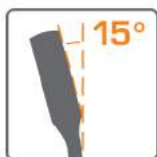
15° offset box end for knuckle clearance.
