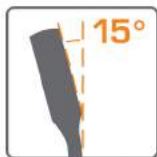
15° offset box end for knuckle clearance.
