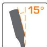
15° offset box end for knuckle clearance.
