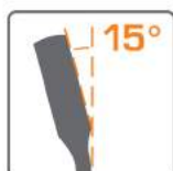
15° offset box end for knuckle clearance.
