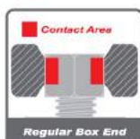
Box end without chamfer increases the contact area with nuts, enhancing the torque of wrench.
