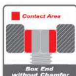
Box end without chamfer increases the contact area with nuts, enhancing the torque of wrench.
