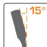
15° offset box end for knuckle clearance.
