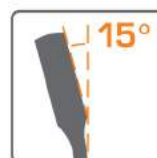
15° offset box end for knuckle clearance.
