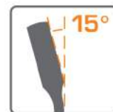
15° offset box end for knuckle clearance.
