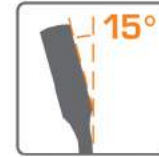
15° offset ratchet head for knuckle clearance.
