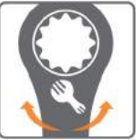
Reversible switch enables wrench to move from either direction.
