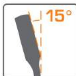
15° offset box end for knuckle clearance.
