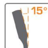
15° offset box end for knuckle clearance.
