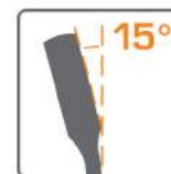
15° offset box end for knuckle clearance.
