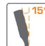
15° offset flare nut drive for knuckle clearance.
