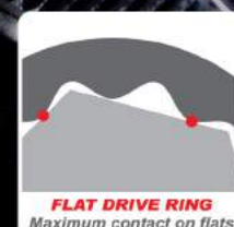
Dual flat drive technology on box end to maximize contact on fasteners.
