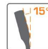
15° offset box end for knuckle clearance.
