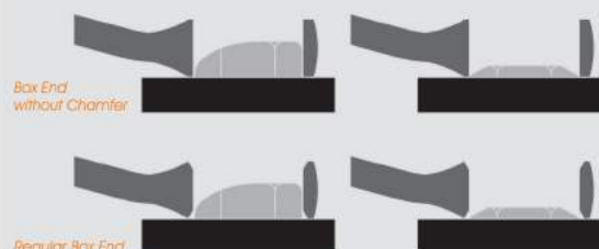
Box end without chamfer fits all types of corrupted nuts.
