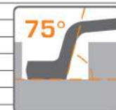
75° offset box end for knuckle clearance.
