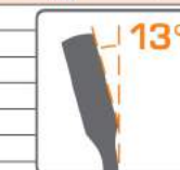
13° offset box end for knuckle clearance.
