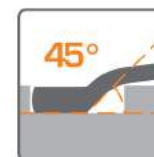
45° offset box end for knuckle clearance.
