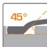
45° offset box end for knuckle clearance.
